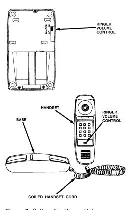
Figure 3. Setting the Ringer Volume Control (Desk and Trimline Telephones)
